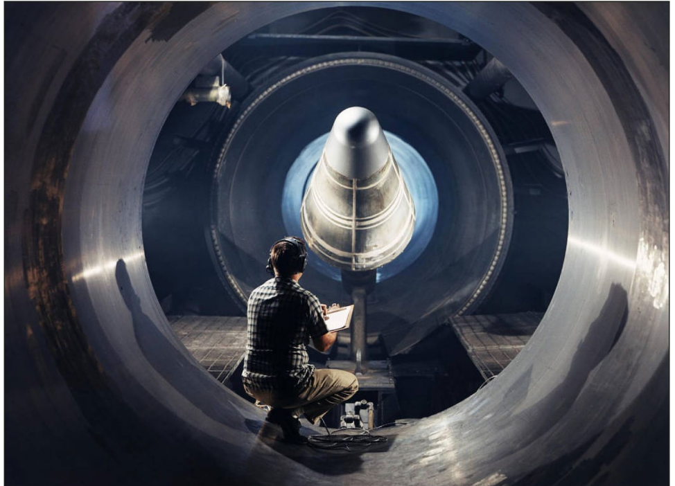
Figure 6: NASA Langley's 8-Foot High Temperature Tunnel Testing a Large-scale Cone Aerothermodynamic Test Article
