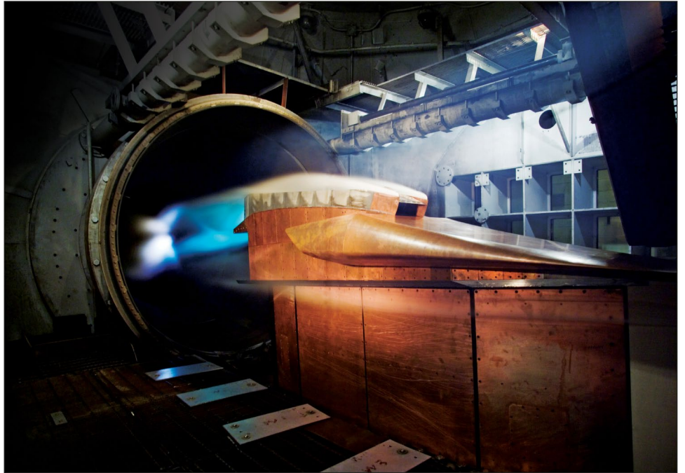
Figure 5: NASA Langley's Hypersonic Model Test in the 8-Foot High Temperature Tunnel
